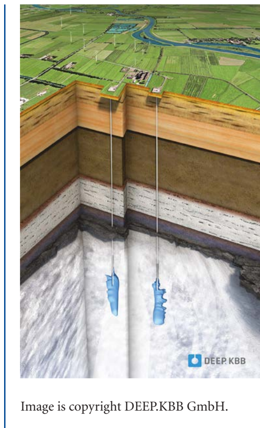
Figure 5.5 Stylized representation of underground salt cavern
