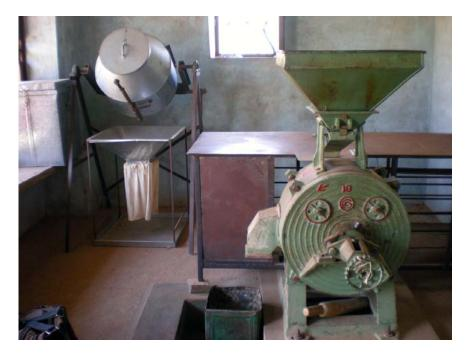
The fortification machine is on the left, and the milling machine is on the right.
